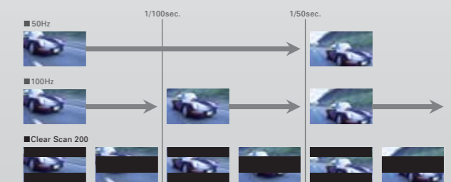
Clear Scan 200 technology scans the picture more often than 50Hz and 100Hz scanning (4 and 2 times, respectively) to produce a picture without motion blurring.
